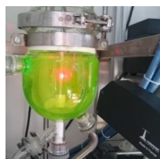
In situ monitoring in a double jacket glass reactor
